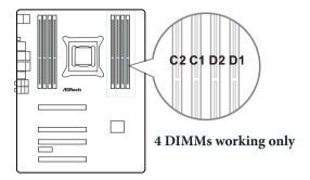
When installing memory modules, the DIMM slots should be populated in the following order: DDR4\_C1,DDR4\_D1 and then DDR4\_C2, DDR4\_D2.
